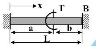
$$T_B = T_i \frac{a}{L}, T_A = T_i \frac{b}{L} \quad (1)$$
