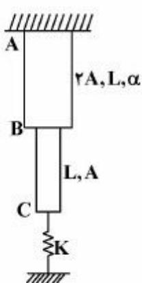
$$\frac{\alpha L \Delta T}{1 + \frac{\gamma K L}{\gamma E A}} \quad (1)$$
