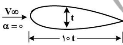
$$R_{et} = \frac{V_\infty t}{v} = 10$$
