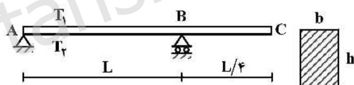
$$\frac{5}{32} \alpha L^3 (T_2 - T_1) \downarrow \quad (1)$$
